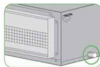
Right drainage hole
